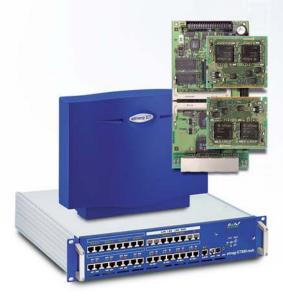
The Gateway module has two slots for DSP expansion modules that expand the gateway to include digital voice channels for Voice over IP. So an elmeg ICT system with VoIP-VPN Gateway becomes a real hub for the entire digital voice communication and allows a seamless transition from traditional voice networks to IP voice data. Every conventional terminal device can use IP voice telephony and ISDN telephony—and conversely each local IP telephone can also be used for ISDN telephony.
