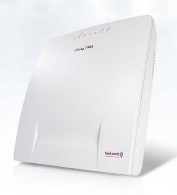
Thanks to the USB port, you can connect your PC to the Internet within a few minutes—and also to an entire Ethernet LAN. The configuration can be performed via USB, LAN, the internal ISDN bus, or from remotely by your vendor.
